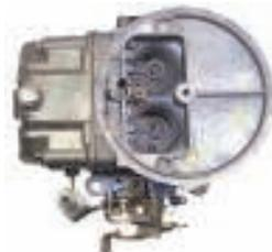
For modified 6 cylinder and V-8 engines that are required to run 500 2 barrels with no restrictions on venturi or base plate size.
