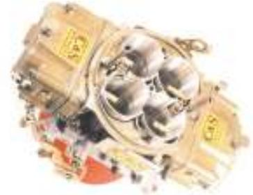
Stock Holley® discharge nozzles are very close to the throttle plates. This creates a fuel distribution problem at part throttle. Throttle plates direct fuel to center of intake manifold. This richens center cylinders and leans end cylinders. Even if total mixture was perfect. This reduces potential torque and smoothness.
